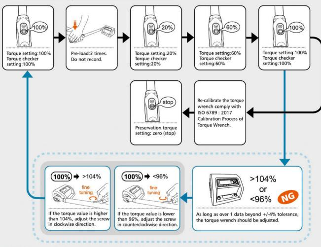
Notice: If the torque data is not in the tolerance (+/- 4%) after adjusting; contact your dealer or send the torque wrench back to factory to do further adjustment.
