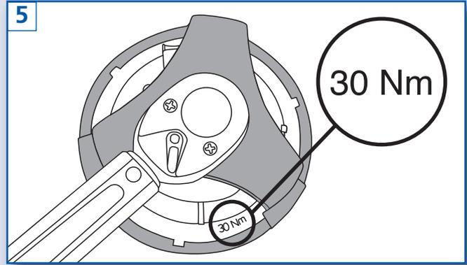
Tighten the fastening ring to 30Nm, then refit the housing to the vehicle and reconnect all fuel pipes and electrical connectors. Start the engine and check for leaks.
