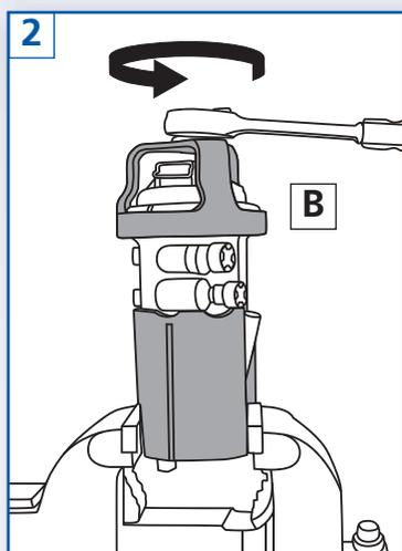
Using a 1/2" drive ratchet simply undo the fastening ring by turning part 'B' anti-clockwise.
