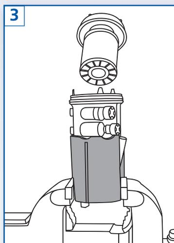
Extract the upper section of the filter housing and replace the fuel filter element (ADK82327) taking care not to touch the filter paper on the new element.
