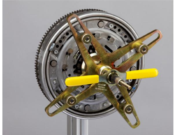
Use the 3-hole pitch on flywheels with six mounting threads, and the 4-hole pitch for flywheels with eight mounting threads.
