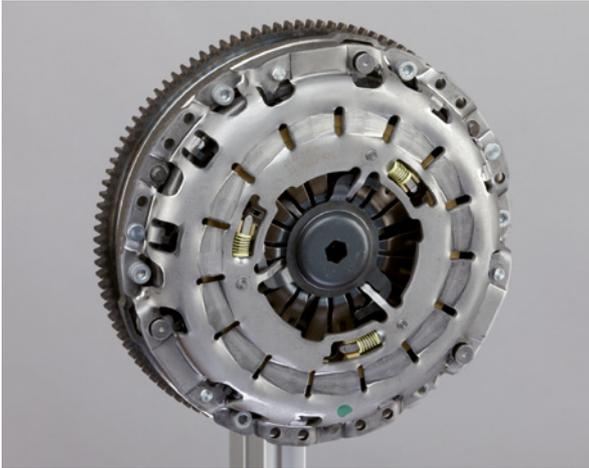
Clutch pressure plates on some BMW models are equipped with a locking device which makes the use of a conventional centring pin impossible. This is why a special pin design or centring sleeve is required.
