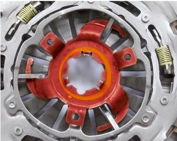
Clutch pressure plates for these models can be equipped with a locking device. The clutch disc is centred by means of the universal centring pin.
