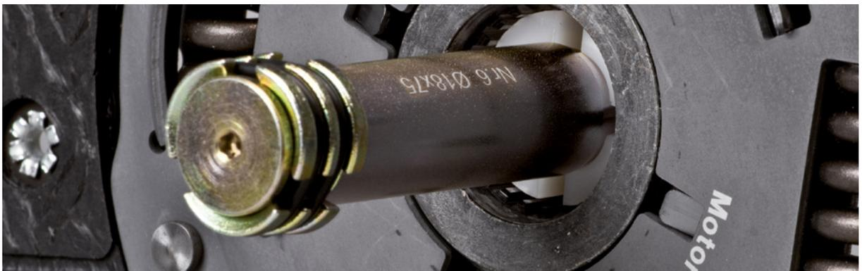
Correct assembly of the centring pin is dependent on the inner diameter of the pilot bearing or crankshaft bore, and on the distance between the pilot bearing or crankshaft bore and the clutch disc's hub profile.
