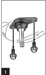
Remove the ball joint bolts.
