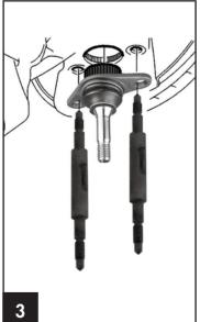
Install the new ball joint loosely using the guide bolts.
