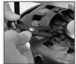
If the old clutch cover is to be reused, it must first be reset. The adjuster ring can be turned back with clutch resetting tool together with clamping tool.
