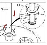
Fig 2: Assemble the handle(B) and the air inlet fitting, turn off the ball valve(H).
