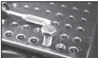
I. When tapping of the hole is finished, from behind the tap, blow chips out with pressurized air. Move the arm on the ratchet to select reverse and slowly back the tap out of the hole, being careful on the last few turns not to catch and damage the threads when removing the tap.
