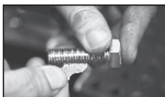
B. Determine the thread pitch using the thread gauge included with the product. The prongs on the thread pitch must fit exactly into the screw thread.
