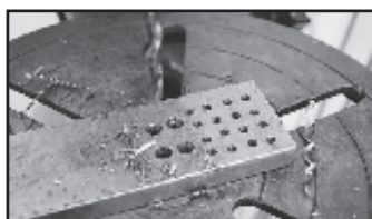
D. Locate or drill your own appropriately sized hole for the tap being used (see chart on page).
