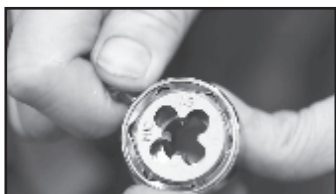
B. Choose the correct bolt die. Insert the bolt die into the die holder. Secure the bolt die using the screw on the die holder.
