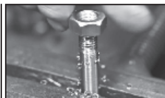
H. Clean the rest of the chips from the threads and check your work with a threaded nut before installing bolt. It may be necessary to apply a small amount of oil or using a fine file to ease the edges of the threads before installation.
