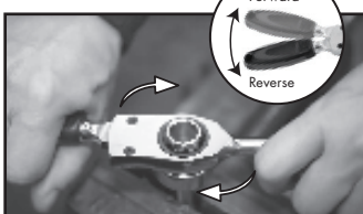
F. Throughout the cut, use the Rapid select ratchet to quickly switch back and forth between forward and reverse to break up the chips for a cleaner cut.
