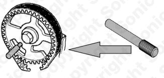
Component 4 - Flywheel Locking Pin (8mm) (1.6 engines)
