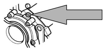
Lock the fuel pump pulley in its timed position with the pump timing marks aligned using **Component 1** as shown.
